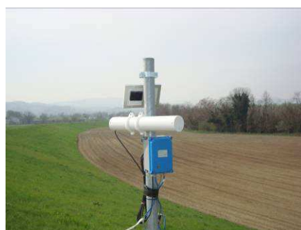
Data transmission system via radio module (Code OD0WL500000)
