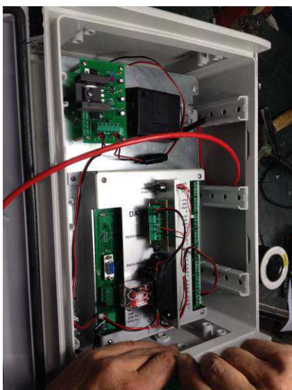
Datalogger D800 (Code OD800C008) Complete with warning system.
