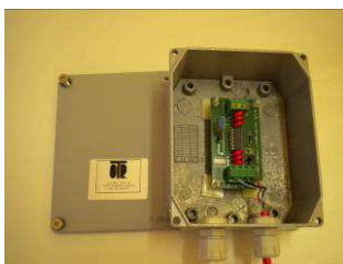
4-20 mA transmitter (Code O00CRK00420) housed in a junction box.
